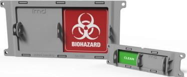
Status indicators are designed and tested to withstand use on cart washers and in autoclaves at 250 degrees for 30-minute cycles without disfigurement or damage. 2-sided mounting tape is also durable in these conditions and can be easily replaced if damaged or for repositioning.
