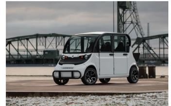
Li-ion vehicles can operate in 35% more weather than AGMs. It is engineered for thermal resiliency in extreme weather with an insulated battery pack that is also heated, which allows for operations in temperatures ranging from -20 to 140 degrees.
