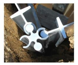
The panels are made of fully extruded 6061 T6 aluminum, and weigh 10lbs. per foot. Panels come in 5" and 8" sections with an effective 16 inch width. Knuckles come in 8 foot sections. Panels stack in a compact configuration for easy transport.
