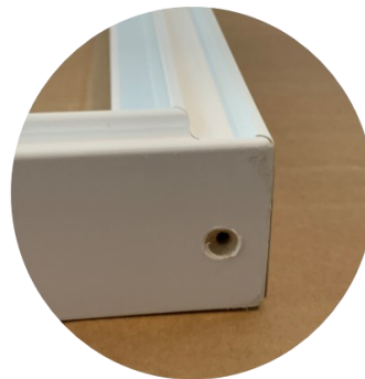
Drill countersink hole
