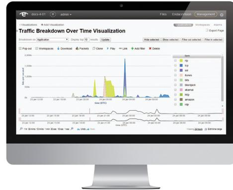
EndacePackets allows analysts to decode packet history directly on the Endace Probe, removing the need to transfer large packet capture files across the network.
