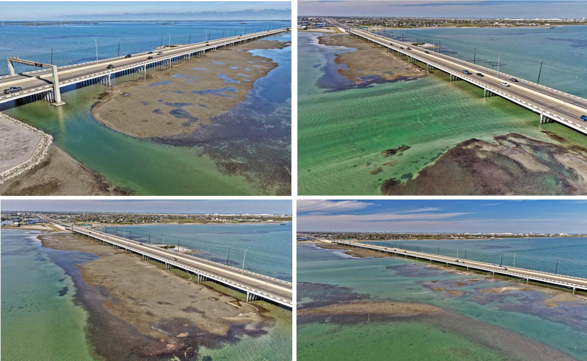
Augs Services got some drone shots of the low water showing the areas along the JFK Causeway where tidal flow is impeded. The low tide revealed the normally submerged sandbars, and the existing channels on the southside of the causeway.
