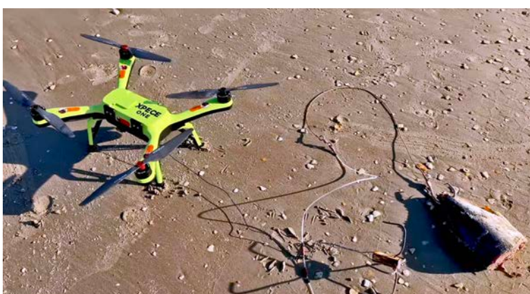
Drones are being produced with large payload capacity for the exclusive purpose of deploying baits for fishing. Here is an example of one of the newest designs.
