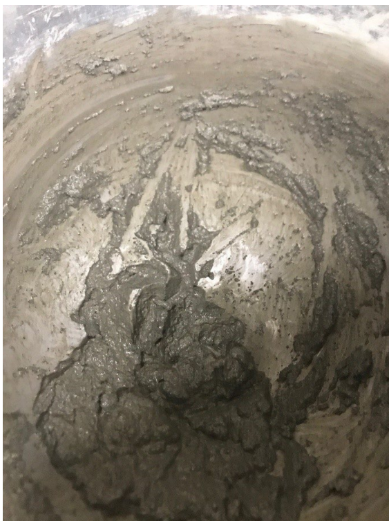
Figure 1: Freshly mixed grout in the mixer
