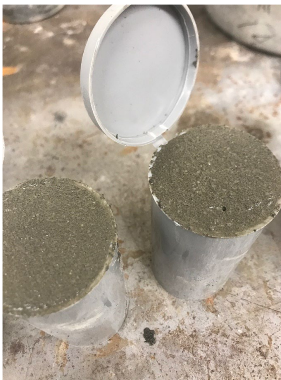
Figure 2: Grout consolidated in 2-inch diameter cylinders
