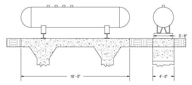
THE DISTANCE BETWEEN THE TANK LEGS (APPROXIMATELY 9 FT.) WILL VARY WITH TANK MANUFACTURER.
