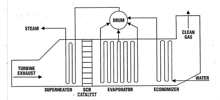
In combined-cycle gas turbine applications, the catalyst normally is placed after the superheater in the heat recovery steam generator (HRSG), where the temperature is in the range suitable for base metal operation (see Figure 3). At several sites in the U.S., hightemperature (zeolite) catalyst has been installed upstream of the HRSG or at the turbine exhaust in simple-cycle applications, where the temperature may be as high as 950-1050 °F.17
