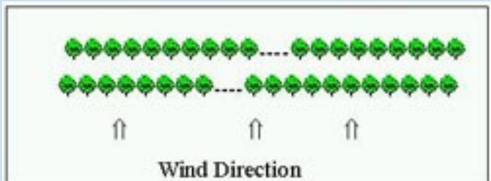
Figure 2. Angling the gap on a shelterbelt can prevent wind tunneling through gateways etc.
