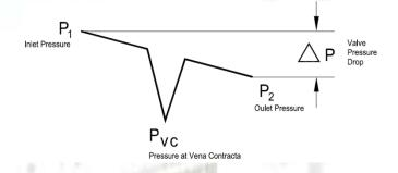
In a single seated control valve the flow travels from P1 (upstream Pressure) to P2 (downstream pressure)
