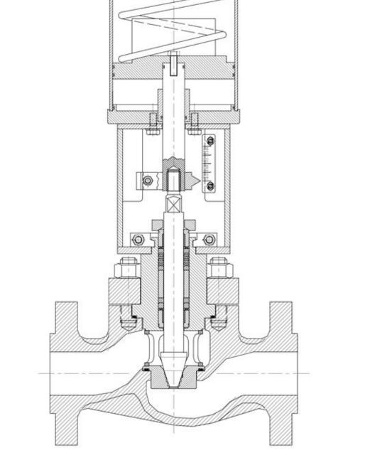
The Delatite Step Trim minimizes cavitation damage in fluids that could contain some solid particles, or low flow situations where small CV values are required.
