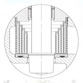
The solution to high flow velocity is to gradually reduce the pressure within the valve without any large pressure drops.
