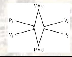
In gaseous applications where there is a large pressure drop across the valve the flow velocity is increased greatly at the valve vena contrata which can generate velocities in the valve which can reach sonic velocity. These sonic velocities can generate high noise and vibration levels within the valve even though inlet and outlet velocities are relatively lower.
