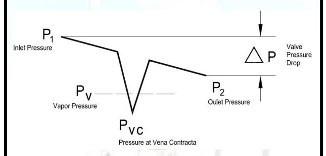
The first stage of cavitation occurs when the fluid pressure drops below the vapor pressure and bubbles form in and around the vena contracta of the valve (seat area) as the fluid continues its path through the valve but after the vena contracta the pressure of the fluid begins to recover.
