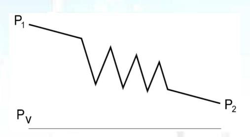
At no stage does the fluid pressure drop below the fluid vapor pressure.
