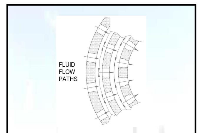
Each stage in the trim have a number of drilled holes which the fluid is forced to travel through.
