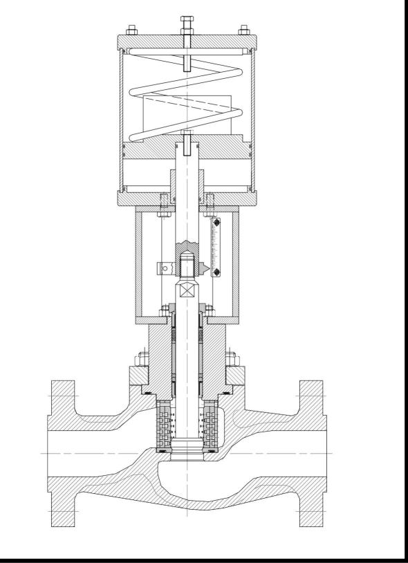
The Delatite Cavitation Control Trim has been designed to eliminate cavitation damage by using a number of drilled hole cylinders and pressure reducing flow passages.
