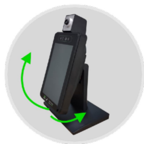
Kiosk with adjustable angle (max. 90°) for various scenarios; supports floor stand and customized options.
