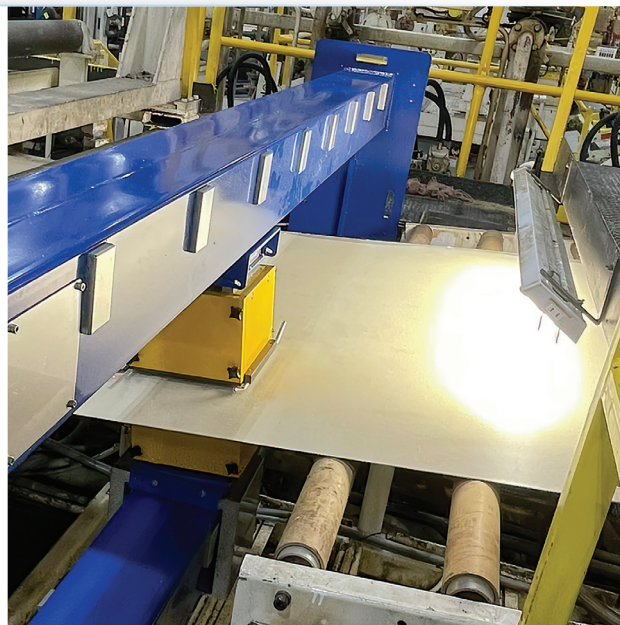
Mikros EMF system installed on a sheet line. The system uses no belts or vector drives and instead relies on an independent linear drive system on each head. The technology is nonnuclear, so no shielding is required. Source: Mikros LLC
