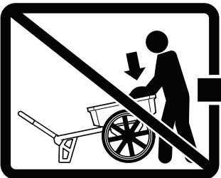
FIG. 3 - TIPPING HAZARD - LOAD HANDLE SIDE FIRST
