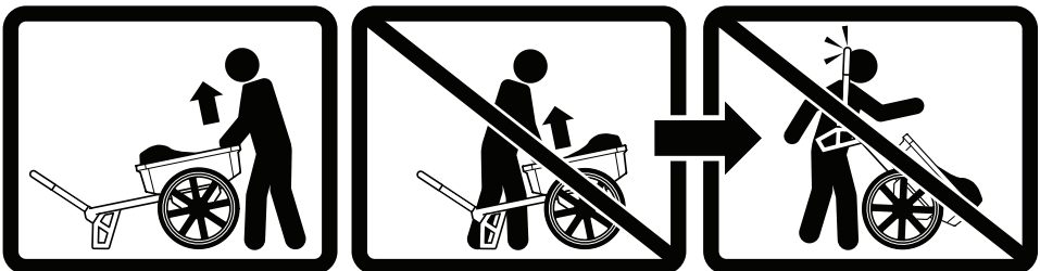
FIG. 4 - TIPPING HAZARD - UNLOAD HANDLE SIDE LAST
