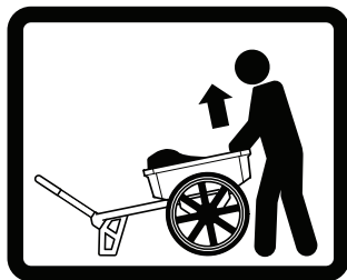
FIG. 4 - TIPPING HAZARD - UNLOAD HANDLE SIDE LAST
