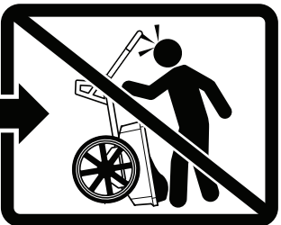
FIG. 3 - TIPPING HAZARD - LOAD HANDLE SIDE FIRST
