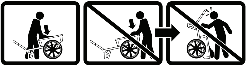
FIG. 3 - TIPPING HAZARD - LOAD HANDLE SIDE FIRST
