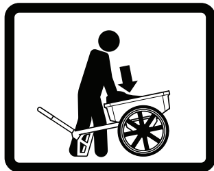
FIG. 3 - TIPPING HAZARD - LOAD HANDLE SIDE FIRST
