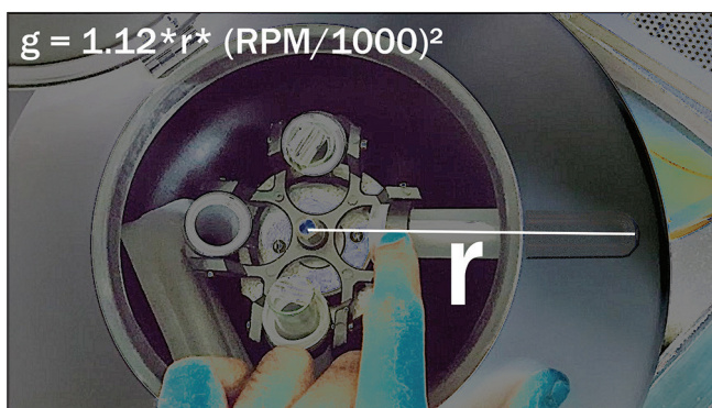
Figure 2: Revolutions per minute and g forces are related by the formula g = 1.12 \times r \times (RPM/1000)^2 where, r is the center of the centrifuge to tube end distance in millimeters
