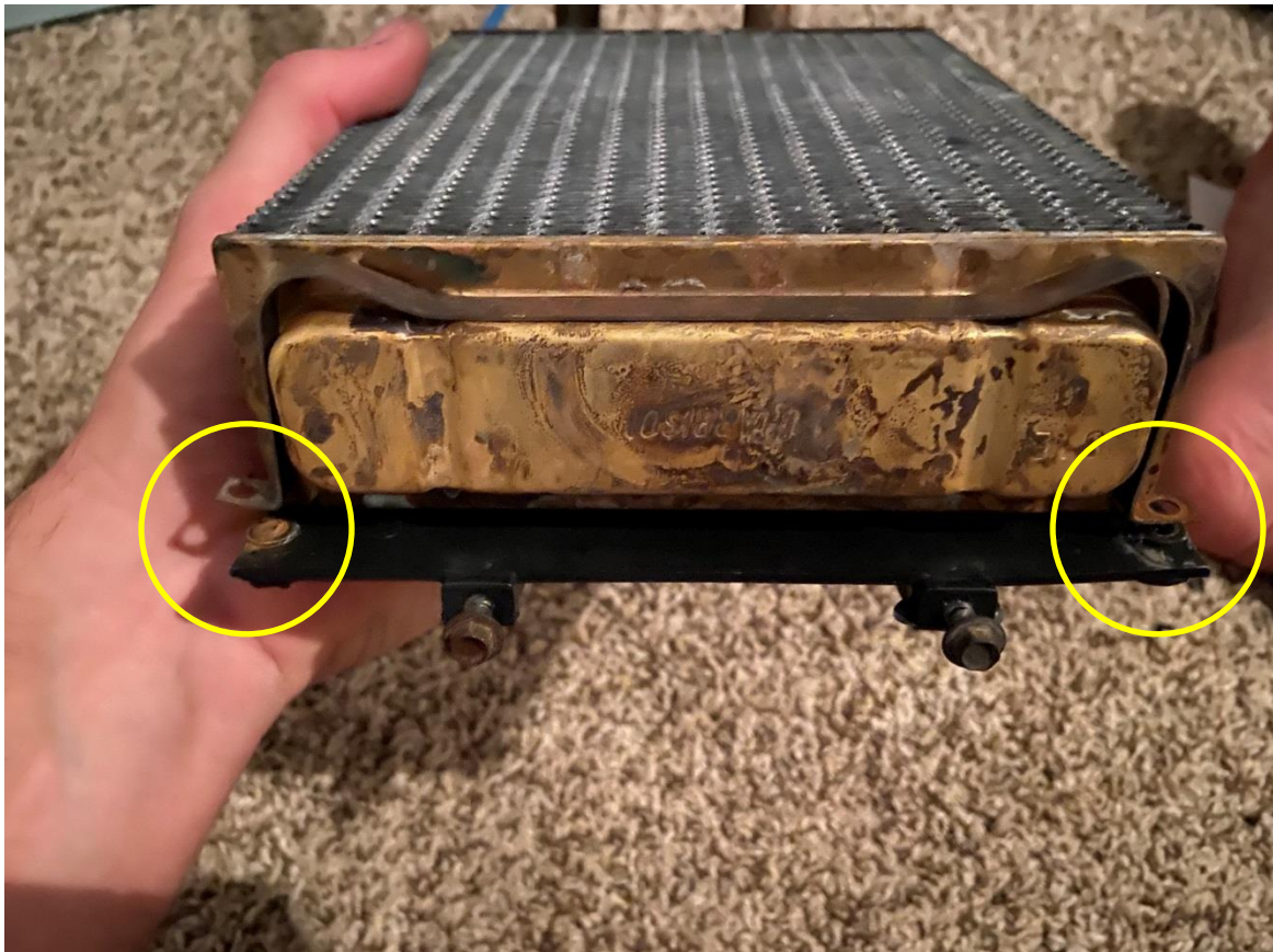
Band clamp is secured on each end with a screw
