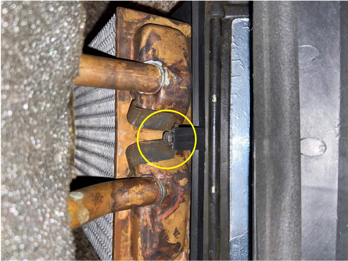
V Clip secured with single screw
