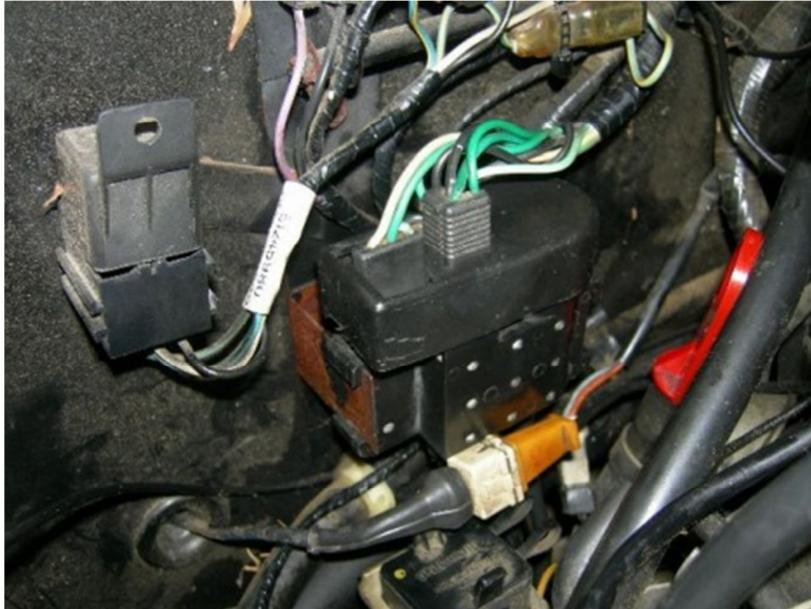
The Connection Box has 5 sets of cables installed on it – two on the top and three on the bottom.
