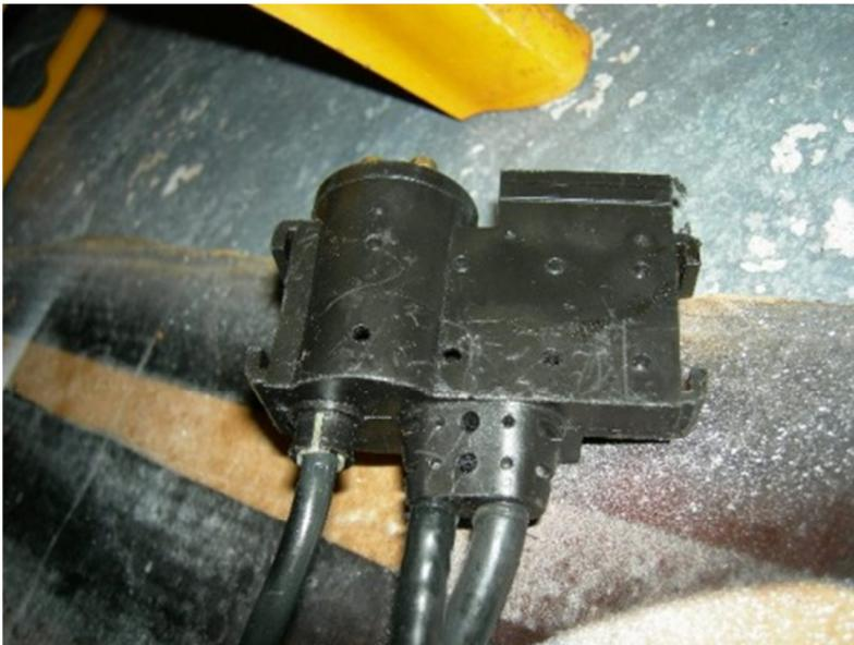
There is one additional 3-conductor cable that enters the Connection Box from the bottom (shown on the left in the above photo), but physically passes through and is connected, via ring-terminals, to three of the brass connectors in the top circle. This is the connection to the solenoids. There is no need to disconnect this cable.
