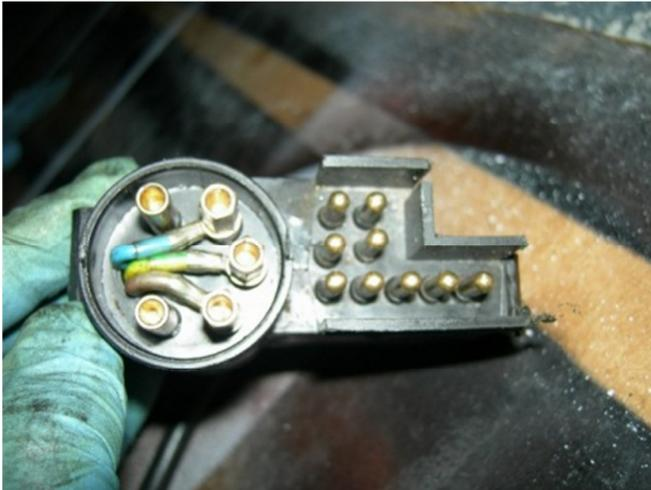
If you are testing the integrity of the solenoids – disconnect the three conductors (by loosening and removing the three 6mm brass nuts (having first noted the colors and locations of the wires) and measure the resistance between the two pairs (Green/Yellow & Blue and Green/Yellow & Brown, the Green/Yellow wire being the common). Each should be around 25ohms.
