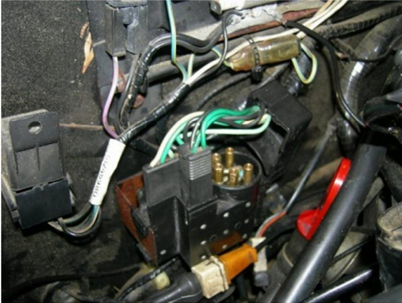
Remove the two L-shaped rubber connectors (to the wiring harness) on top of the Connection Box..
