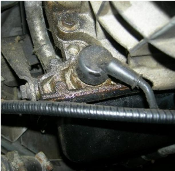
Remove the transmission pan. It is attached by 11mm bolts. Remove pan and gasket (use a new gasket for reassembly). At this point it is worth inspecting the pan for debris which may be indicative of a transmission problem. The filter can also be inspected.
