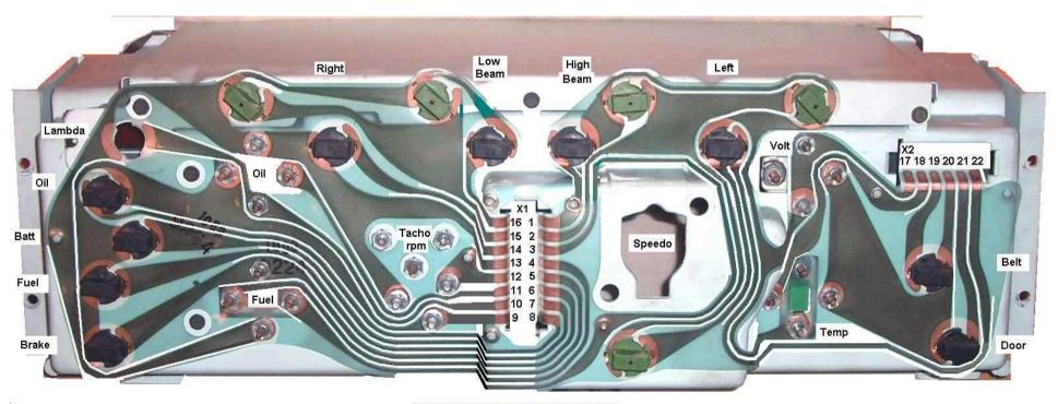
The numbers on the connectors match the car's schematic.
