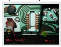
The first job is to remove the speedo cable connection. Pushing the clip back towards the rear of the dash at the same tune pulling the speedo cable off. As shown in the picture.
