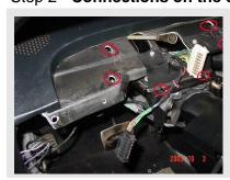
The binnacle itself has 6 threaded posts which go through the holes as shown.
