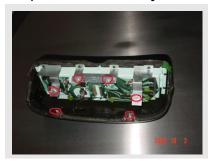
The dash binnacle is secured by (6) 7mm nuts, 3 on each side almost symmetrically located. These nylon/metal nuts each have a washer, The two towards the center have smaller washers.
