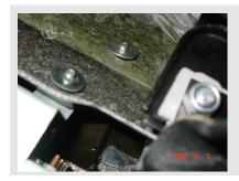
Here is a view of two nuts on the center side from under the dash. These will be removed with the 7mm socket and wrench with the flex attachment. The third at the steering column is not visible in this picture.
