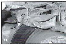
Using a straight edge screwdriver, turn the adjustment bolt clockwise to locate the parking brake pads against the rear wheel disc (Photo 12). Back off the adjustment bolt 1/2 to 1 turn, and replace the cotter pin.
