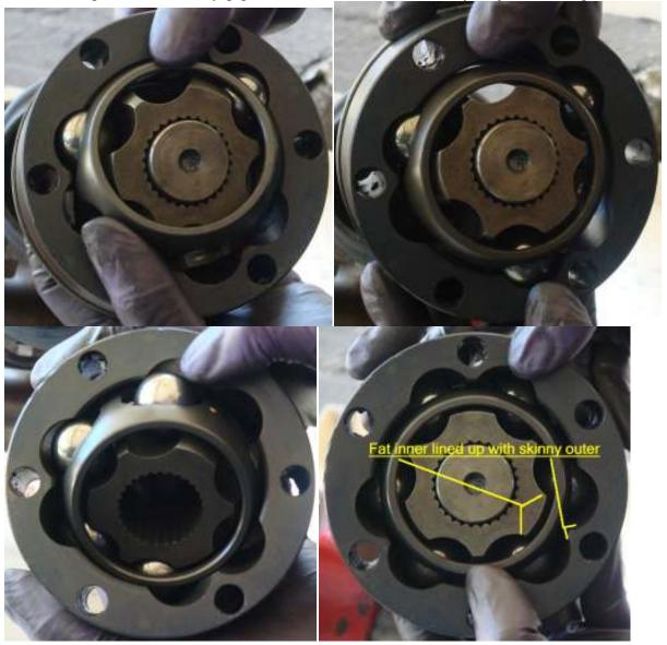
Step7: When reinstalling your assembled joint be careful not force it on to hard without securing the inner and
