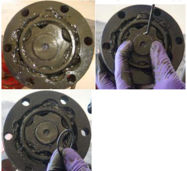
Step4: Now you can remove the joint from the shaft, being careful to secure both the inner and outer races so as to not allow the joint to disassemble. Go ahead and remove the old boot, clean the shaft end and install the new boot.
