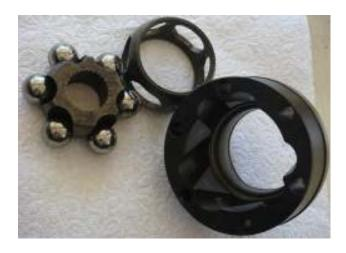
Step6: Reassembly can be tricky but not impossible with some patience. You may prefer to reassemble with the joint on the shaft or off, I prefer off but start out with it on in this example. Reassembly is more of an art than science and trying to explain "the" way of doing it is probably impossible so I will leave it at this: get one bearing in at a time and work the inner race back and forth as you reinstall the bearings one at a time.
