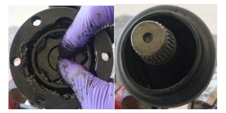
\*\* How you choose to clean your joint will dictate how you approach this next step. 5a will cover the easier of the two methods but requires more time than 5b. 5b allows you to do a thorough inspection of all the joint components but reassembly of the joint can be tricky. Personally I prefer 5b because it is. IMO, faster and does not leave me with a bucket of dirty cleaner that I don't know how to dispose of.
