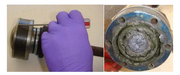
Step3: Wipe off the surface of the joint to expose the snap ring. Using either your mechanic's picks or snap ring remover, remove the ring. Be cautious here to not allow the ring to shoot off as it can and may injure!
