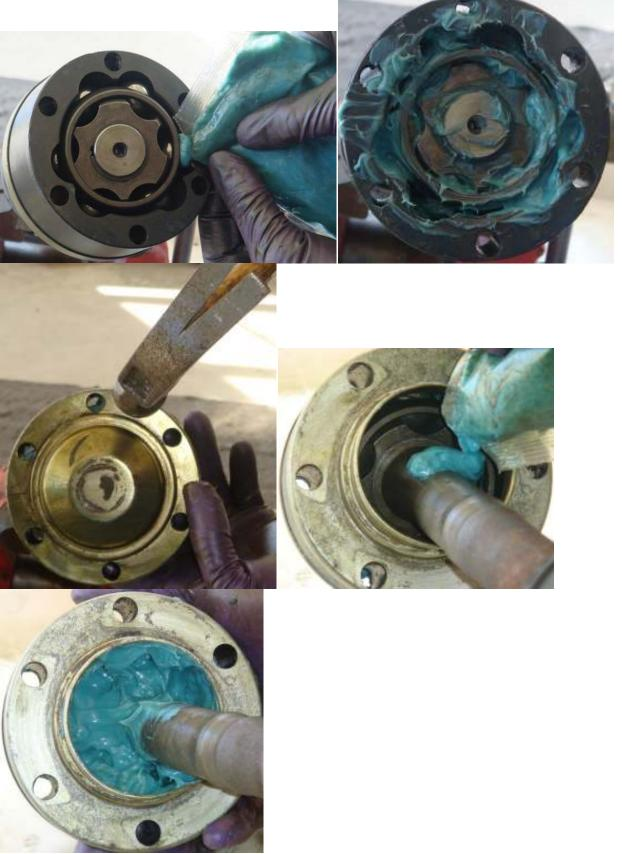
Step9: With the joint repacked you are ready to slide the new boot over the joint flange and clamp. Depending on the style of clap that comes with your kit you may need special pliers to finish this process. The kit used on this How-To came with wide heavy duty zip ties and are secured using regular needle nose pliers and a knife to trim back the excess.
