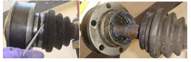
Step2: With the screwdriver and hammer, lightly tap off the joint cover plate to expose the joint.
