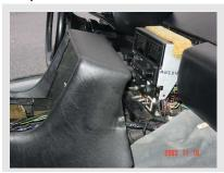
At this point, it may take some work lifting and pulling (towards the rear of the car), the center console will come up and back off of the heater duct.
