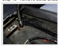
Remove the 2 10mm nuts and washers on both sides , directly under the power window switches.
