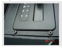
Remove the two phillips screws as shown.
