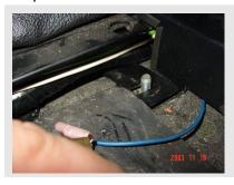
Remove the two 10mm nuts and washers to the left and right of the arch shown below. (Where the wires go through) (Left side shown)
