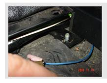
On the driver side, lift the forward bracket up off of the post and get the cables running along the metal bar UNDER the bracket. Do the same with the other side
