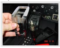
Remove the metal piece and the spring. Watch that the spring doesnt shoot away!!
