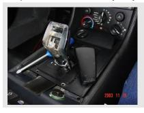
Remove the top black cap to expose the nut and washer. Remove the nut and washer.
