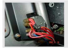
Remember where the wires go to on the brightness adjustment switch (4 connections) and remove them.
