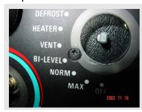
A small phillips screw holds the display cover in place. Loosen the screw and pull the cover out from the top first. Then stick your hand behind to pull the the light sockets off of the back for the FAN FAIL, the DOOR LOCK and the REAR DEFROST.
