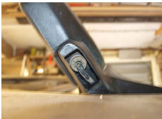
The appropriate tension to the mirror is applied by a sequence of 6 washers that when compressed by a 7th star lug nut (washer), provides the mirror with the capability to hinge when subjected to slight impact (ouch!) yet not flop about when driving on uneven roads. (see later photo showing the shape and sequence of the seven washers on the pivot tube).
