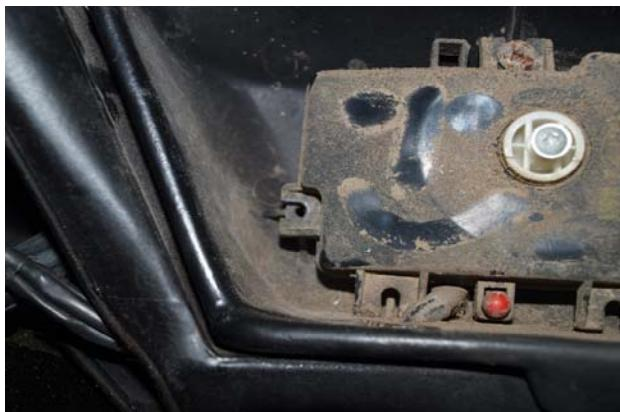
The loom o the mirror (the wires that run through the pivot tube) is uncoupled within the recesses of the
