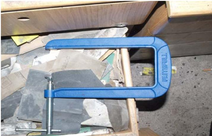
So I came up with the idea of using a G clamp as a press. The above shows "Old Faithfull" - I'd bought this to clamp down the roof box while I bolted it down. The wide mouth of the clamp enabled me to hold the clamp between my knees when I pressed on the Star Lug - otherwise a second pair of hands would probably be required.
