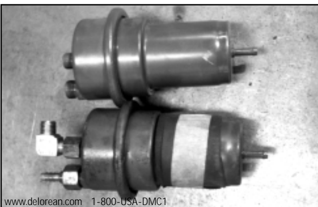
Figure C – new fuel accumulator positioned top of picture. Old fuel accumulator with fittings and black pad still attached positioned bottom of picture. Remove fittings and pad from old accumulator and place on new accumulator in same position.
