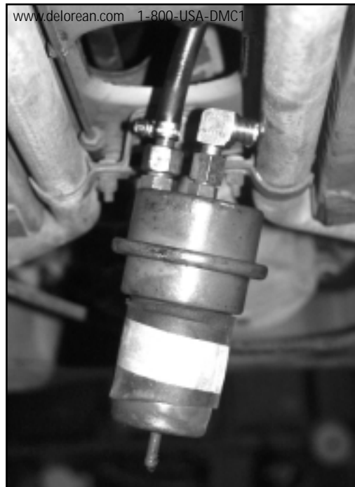
Figure B – Pull the fuel accumulator through the hole in the underbody so it is hanging loosely.
