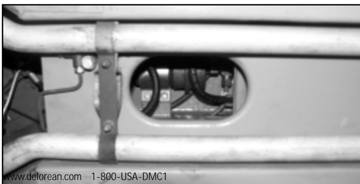
General location of Fuel Accumulator for removal. Old accumulator in place.
