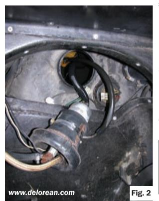
sharp razor blade to cut the old hoses from the barbed fittings in at the frame, leaving the metal ends exposed.
