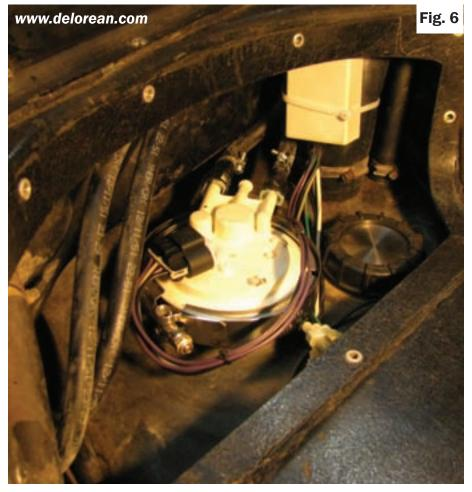
will be stopped by the car body. Tighten the large clamp firmly, but not so tight you break the pump housing! It needs only to be tight enough to keep the pump from rotating.
