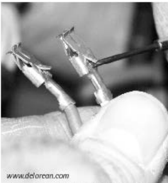
Figure D - Properly positioned depression tab.
