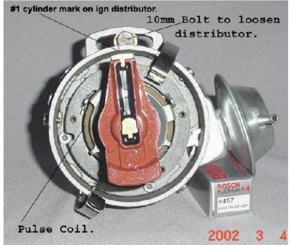
Photo courtesy of John Hervey. Again, the worm gear may cause it to rotate clockwise as you push it down. If it does, remove the distributor and rotate
