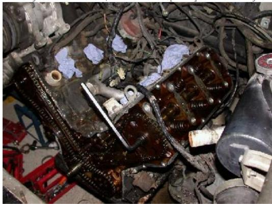
Remove the 10 mm allen bolt from the cam sprocket. Make sure you're not bending the timing chain cover and the cam is backing out of the rear of the head if you are using the support bracket. The manual instructs you to use a metal object and hammer to tap the guide pins (locating roll pins) down flush with the engine block. Mine were rusted and wouldn't depress.
