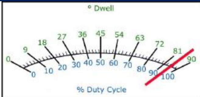
Lean Condition, Rich Correction
