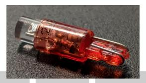
Bend both of these little wires and straighten them, then snip off the excess so that they do not wrap around the base.
