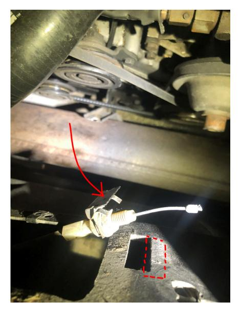
11. Here you can see that you have to remove the rightmost nut from the cable tensioner to be able to remove the clip. I put the clip back where the red dashed box indicates. Then I put the nut back on the tensioner to not loose it. After that you can pull the cable out of the fascia.
