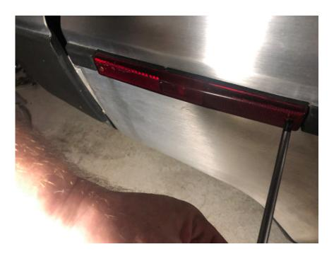
1. Start by loosening the rear side marker lights to be able to pop the bulb and wire out of its holder. All that is required is a small Philips screw driver.
