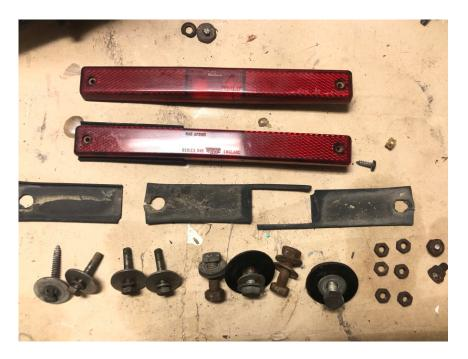
These are actually all the nuts and bolts required to be removed to be able to pull the rear fascia off the car. Not too bad.
