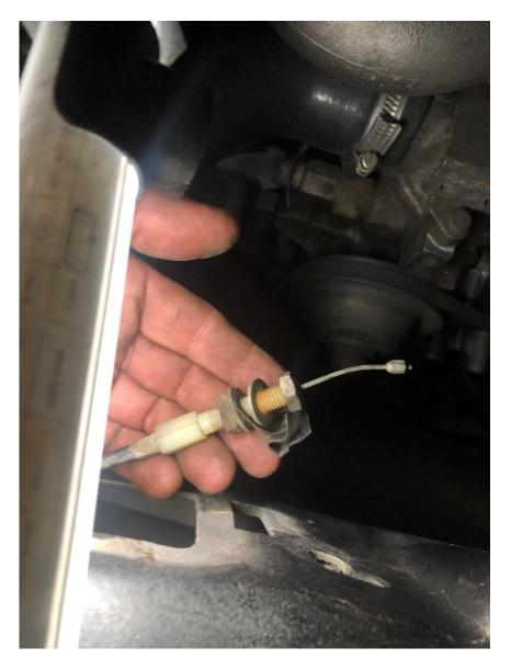
10. By tilting the cable in the lever you can easily pull the cable-stop out of its groove (inside the fascia). I found it easer to first completely remove the tin clip which holds the cable tensioner to the body. The clip is the black, bent metal part hanging on top of my middle finger. You then need to undo the end nut (the rightmost one) to take the clip off, to be able to pull the cable through the fascia later.
