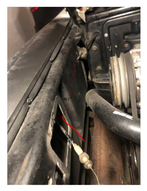
12. The red line in this image shows how the cable runs inside the fascia and out through a grommet in the rear driver side corner of the engine bay. The grommet is easily loosened, and then you can pull the cable and tensioner through.
