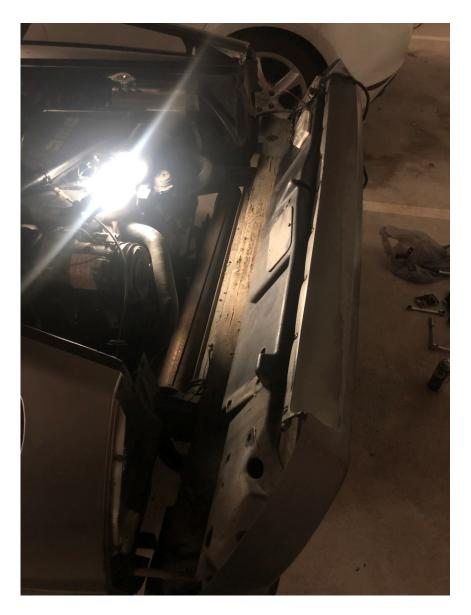
19. When all bolts are removed, you can pull the fascia straight out (backwards) and lift if off the car. Make sure you have separated the studs att the bottom of the fascia from the muffler bracket. You will have the complete wire loom still attached, with the wires for the rear lights, the side marker lights and the black connector for the bulkhead.
