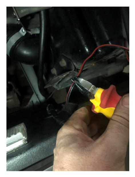
18. This just shows me having to cut the wire to my third brake light which connect to the brake light in the rear light board. I had made the third brake light removable by installing a connector at the top, should I have to remove the Louvre, but I didn't plan for removing the rear fascia. I will install a connector here as well when I assemble everything.
