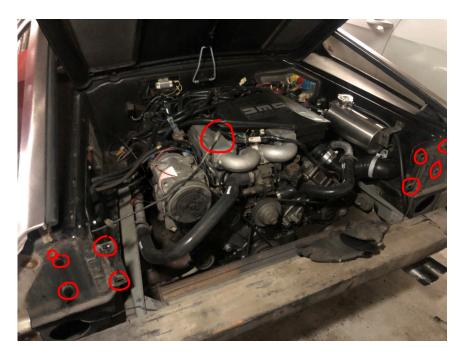
20. Here is an image showing the engine bay without the fascia, and I have marked where the bolts attach. On top of the engine is the cable for the engine cover latch.
