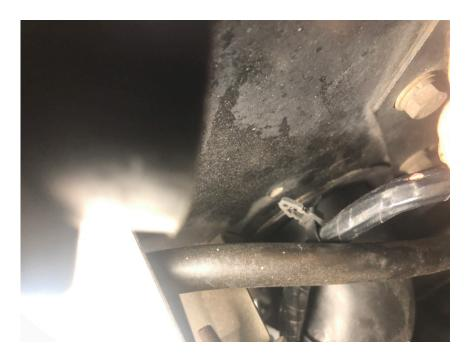
7. On the second clip I used a small flathead screwdriver to press down on one of the tabs, so I could pull it out without damaging it. The clip is the little arrow-head looking plastic piece on the cable tie on the loom. It is pointing straight at the tiny hole where it was attached.
