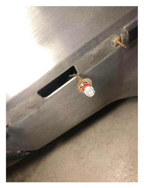
3. With the bulb now hanging free, just pop it back into the hole in the stainless panel. The wires connect to the fascia harness and are easily pulled out once the fascia is loose. You need to do this for both sides.
