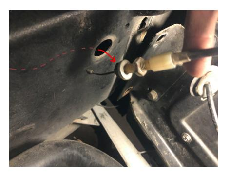
13. Here I have pulled the wire and the tensioner out through the hole ni the fascia, and then I just placed it on top of the engine. *Remember to keep track of it if you intend to start your engine, it can easily get stuck in the belts!*
