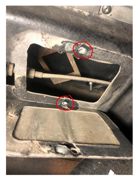
9. Here you can see the cover opened, and the cable runs behind it and is attached to its lever just to the left of the nuts in the picture. The odd metal frame hanging behind the cable is supposed to hold one of the license plate lights attached, but someone put speed nuts to hold mine instead.
