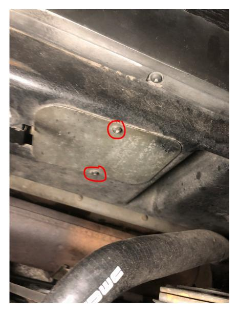
8. Next, you need to loosen the cable which unlocks the engine cover. The latch cover is on the inside of the body, behind the license plate. It is held by two small Philips screws, and I also had to pry the cover loose due to some gasket material which had stuck fairly tight to the fiberglass. You can see the two small screws holding the cover in place circled in red.
