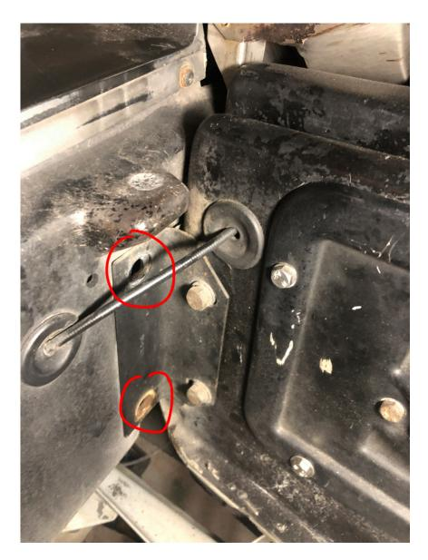
15. Here are the holes in the L-shaped bracket on the inside of the engine bay (*driver side*) where the bolts came through and where the 13 mm nuts were attached. Technically, you could probably just as well loosen the *other* two bolts in the L-bracket, the ones that goes into the fiberglass body, instead, but I choose to leave the bracket on the car, and therefore loosening the two bolts that run from rear towards the front instead.
