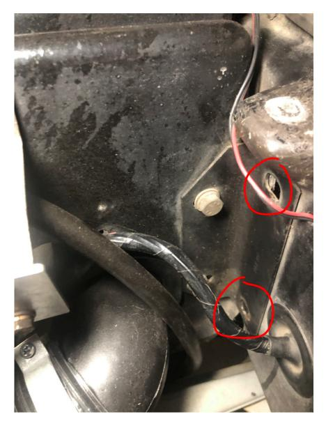
16. Here are the same holes on the inside of the engine bay but on the *passenger side*. The 13 mm M8 bolts came through here and were held on by two 13 mm nuts. You can also see the black wire loom that will be removed with the fascia, after you have disconnected the black connector from the bulkhead behind the coil cover. The whole loom will be removed with the fascia, there is no need to loosen the rubber grommet you see in the picture.
