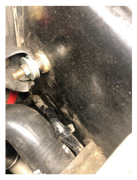
5. The wire loom is fed along the fiberglass body and under the overflow bottle. It is attached in two places ty cable ties with tiny clips on them. The clips are pressed through small holes in the body. This and the next picture shows how one broke when I pulled it out.
