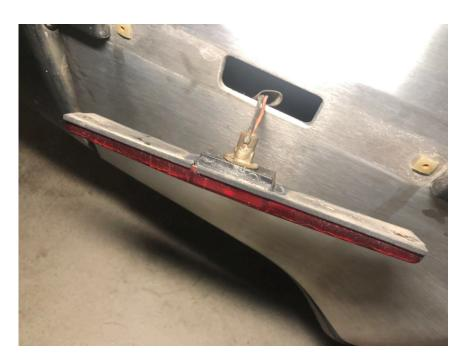
2. Once the lens is loosened, you pull on the bulb to get it out of the socket. I screwed the small self tapering screws back into their plastic nuts to not loose them. If you need to replace the plastic nuts, the bulb sockets or the gaskets, they are available from <u>Deloreango.com</u> (<u>http://www.deloreango.com</u>) and others.
