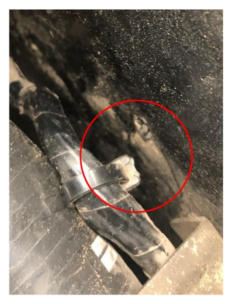
6. There is the broken cable tie which attached the wire loom to the body. The clip is still inside the little hole.
