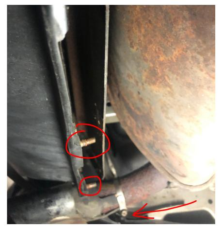
17. When the bolts behind the tail lights are removed, you need to get under the car. This picture is taken underneath the car facing up. The big rusty part on the right is the muffler and also shown at the bottom of the image is the driver side tail pipe. Circled in red are three of the M6 studs that hold the fascia to the muffler
