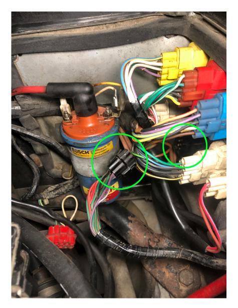
4. To be able to pull the harness with all the tail and side light wires away with the facia, all you need to do is to loosen the black connector in the bulkhead. Remove the plastic box covering the ignition coil to get to it. The connectors are held on by two tabs which you press together with your thumb and index finger and then pull straight out. A good time to clean all contacts.
