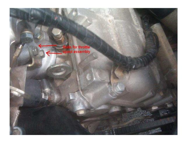
**Step 8:** Remove the fuel mixture unit
