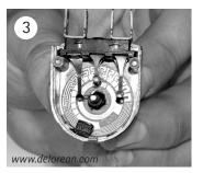
when removing the wires from the terminals, as excessive force can break the terminal block, of which there are no replacements available.
