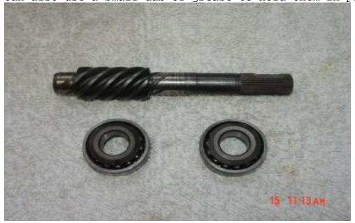
Next, holding the pinion upside down from how it is installed on the car, slide the top bearing over the fluted shaft part of the pinion and hold it in place. I used a wrap of electrical tape on the shaft of the pinion after I had slid the bearing on to hold it in place and then removed the tape after I had installed the pinion and bearings in the housing.
