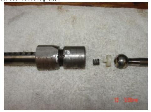
THIS IS A KEY ITEM!!! That large nut is really two (2) jam nuts that are friction locked on the steering bar, just like the tie rod ends are held in place by a jam nut. They are backed up by the use of a "pin" inserted into a hole that is drilled between the two nuts and peened into place.
