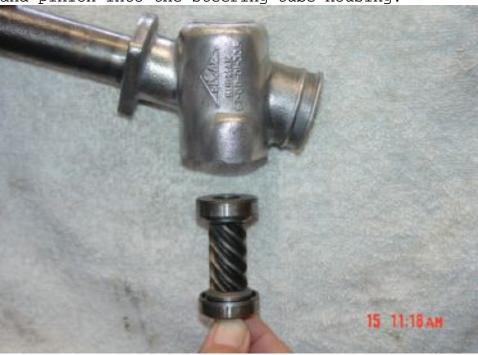
A bit of 90W gear oil coating the outside of the bearings and the inside of the pinion housing will help with installation.
