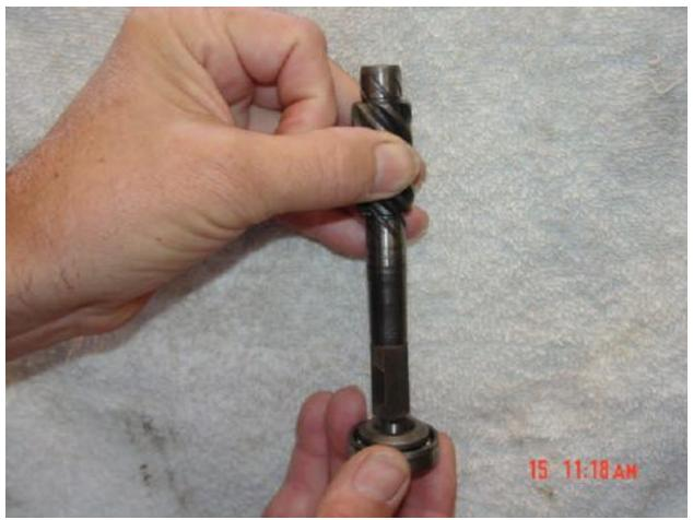
Then, slide the lower bearing on the pinion and let gravity hold it in place.
