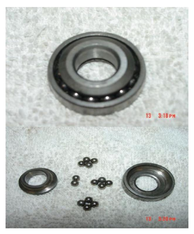
Step #5---Clean all parts and replace any that are bad. Note: The pinion, the bearings, and the steering rod are made of hardened steel, so they very seldom are bad. There is just not enough force or pressure on them to override the hardness of the
