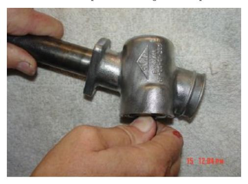
Once you have it fully inserted, turn the steering tube right side up and remove the pinion and upper bearing being careful not to pull up on the lower bearing, spilling the balls all over the inside of the pinion housing. Now, carefully slide the
