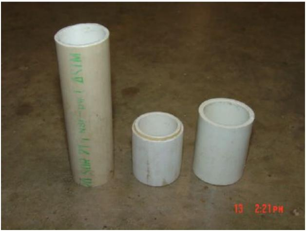
Starting with the two outside pieces in the picture, I took a 3/4" PVC union (outside diameter 1 and 5/16") and cut it to the 1 and 1/4" length. I then sanded the inner bore of this to be smooth so a piece of 3/4" PVC thin-wall pipe would just start to slide in. I used thin-wall because it had an inner diameter of 7/8" and fit perfectly over the steering rod.
