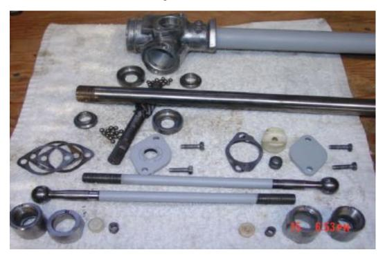
One rebuilt and refurbished Delorean Steering rack awaiting new boots and tie rod end covers is shown below.
