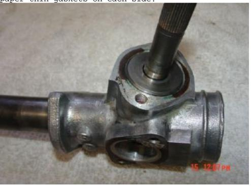
Step #2---Install the plastic retainer and the spring and the oil refill cover, but just snug the bolts down, don't torque them to specs. You will see why later.
