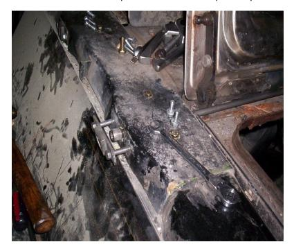
On the driver side the torsion bar should slide right out. On the passenger side it may well be cockeyed and stuck in the hinge. If the bar is cockeyed and stuck in the hinge, break it free by rotating it towards the driver's side of the car. It will make the worst sound you ever heard when it lets go -- sounds just like the bar breaking in two.
