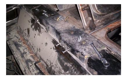
Slide the retaining bracket back onto the long bolts. In some cases you may need to use a puller.
