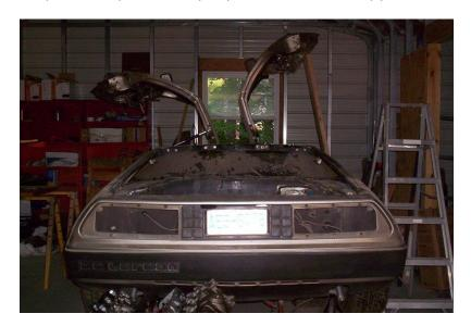
\*ONE AT A TIME\* replace the retaining bracket bolts with long 8mm bolts. This will ensure the retaining bracket can't rotate and hit the back window, no matter how much torque is on the bar (if the bar is torqued normally, there should be virtually no torque with the door propped past vertical).
