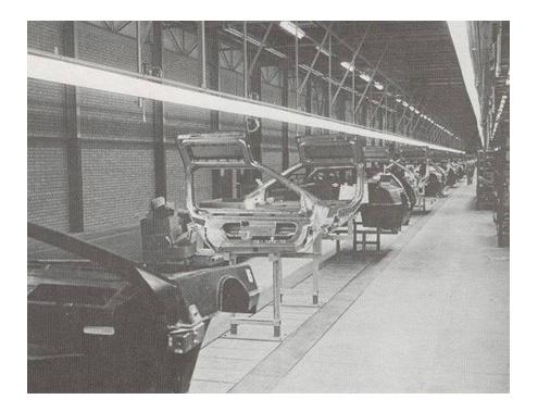
Pages 254-267 of "Celebrating the Impossible" clearly illustrate that doors were attached to body tubs and adjusted/torsioned, to "proper operation" on a separate sub-assembly line. They were then transferred, by overhead crane, to a Tellus carrier for the remainder of the assembly process (body panels and most of the interior were installed \*AFTER\* the doors were working properly). Also visible in this pic. All we're doing is replicating the original factory torsion bar process.
