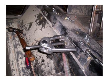
Bracket off the bar. At this point there is absolutely no torque on the torsion bar.
