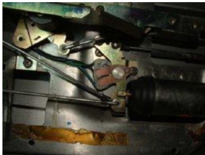
Figure 4: Bellcrank switch UNLOCKED.
