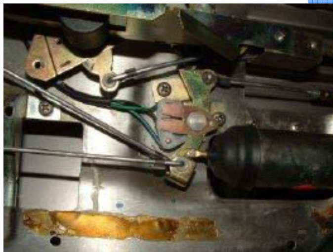
Figure 3: Bellcrank switch in LOCKED position.
