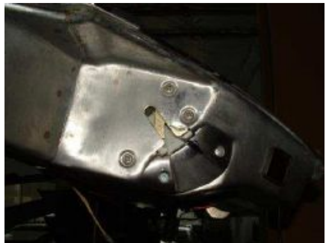
Figure 2: Latches shown normally OPEN.
