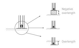
Positive overlength is possible up to the maximum passage height (9' 6 11/64") plus 1' 7 11/16" (11' 1 55/64"). Negative overlength is possible up to the minimum passage height [1' 7 11/16"].
