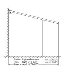
A shifted column in Lapure must be entered by entering the required distance from the wall connection. Minimum shifted column position = Projection - 3' 3 3/8" Maximum shifted column position = Projection - 5 29/32"
