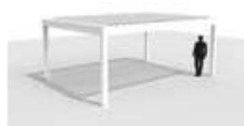
Freestanding: the frame of the Camargue is supported by four vertical columns
