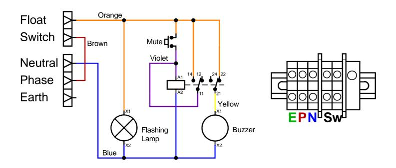
High level alarm, low level alarm float switch wiring
