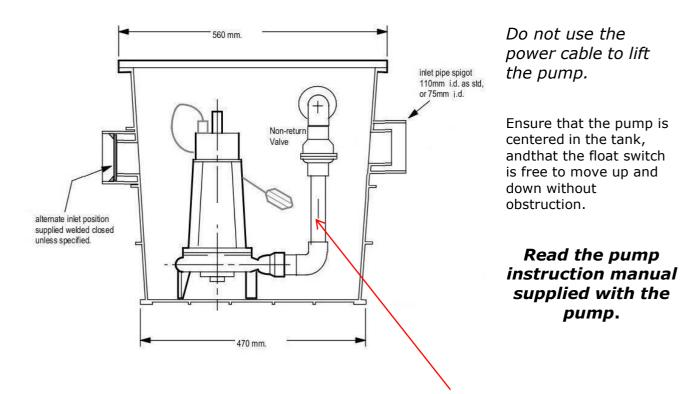
This pipe is not glued. Cut to suit, then glue and test.
