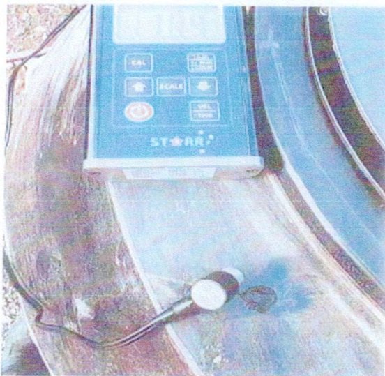
Photos 3 and 4: Material thickness testing. Base, sidewall and top all well in excess of 10mm wall thickness.
