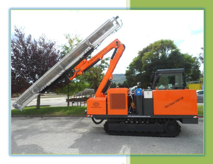
Solar Cleaner C4000 Telescopic is the last model of photovoltaic panels cleaning machine realized by B.P. Metalmeccanica.
