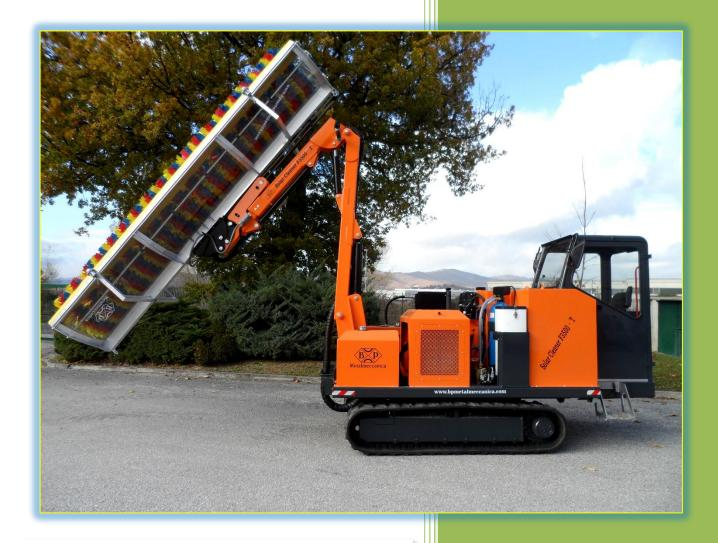
Solar Cleaner F3500 Telescopic is the last model of photovoltaic panels cleaning machine realized by B.P. Metalmeccanica.
