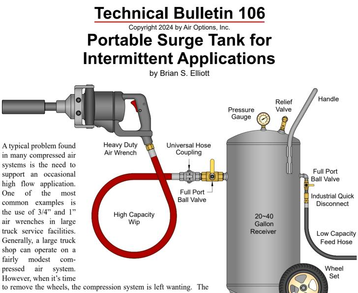
heavy-duty air wrenches simply can't be adequately supplied with a small air compressor and under-sized pipes. In an effort to compensate for this deficiency, many shop owners feed full output pressure to the distribution system (175 PSI). While this does help, it can also have a damaging effect on the internal components of the wenches.
