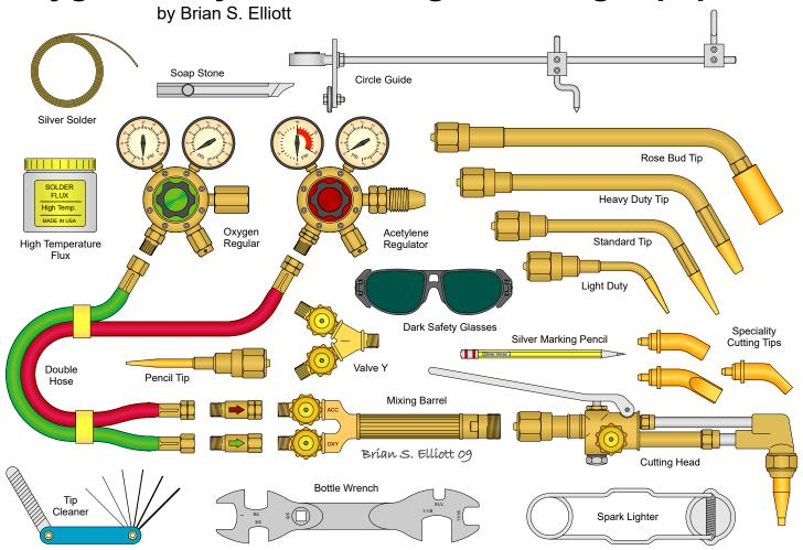
Oxygen and acetylene welding and cutting sets represent one of the foundational tool sets in the typical steel fabrication shop. Commonly referred to as "gas welders" or "cutting torches", these sets are astoundingly versatile pieces of equipment. They can quickly cut through a 10" thick piece of steel plate and minutes later, be reconfigured to solder miniature instrumentation components. The impact that they have on metal fabrication industries is virtually incalculable.
