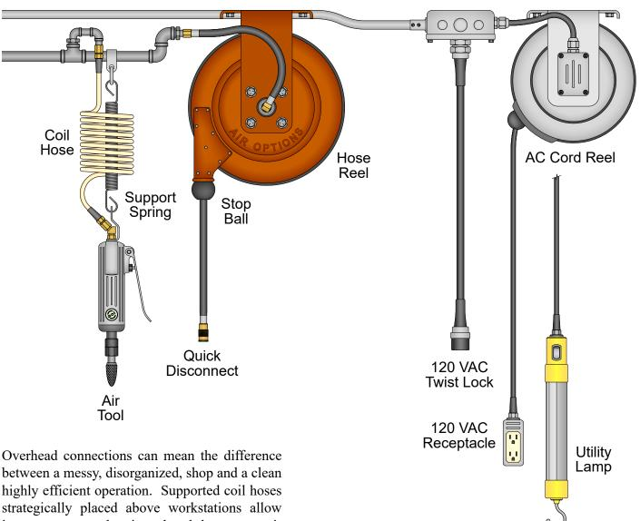
between a messy, disorganized, shop and a clean highly efficient operation. Supported coil hoses strategically placed above workstations allow instant access to the air tool and they automatically return to their storage locations when the operator lets go. Hose reels provide quick access to compressed air and electrical applications. Additionally, they can be stowed in their home position nearly as fast as they can be deployed.
