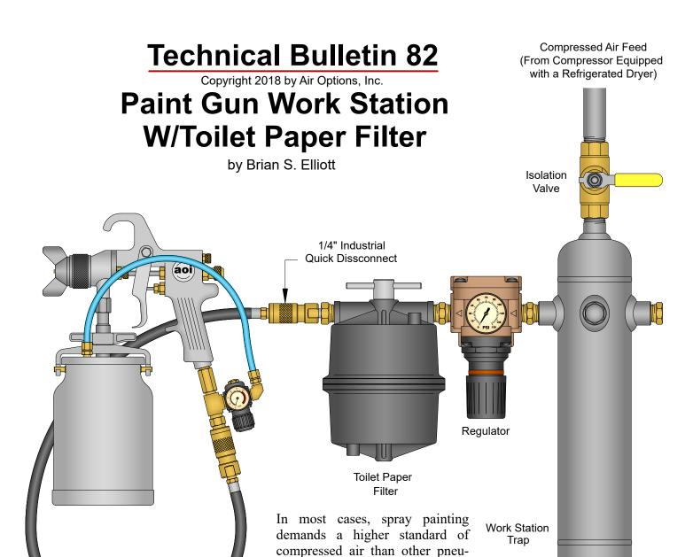
matic operations. A simple, effective and inexpensive paint gun work station can be set up as shown in the illustration. An arrangement like this can dramati-
