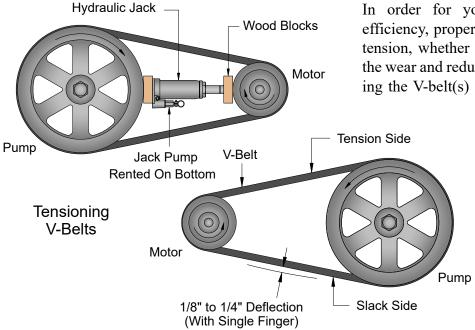
In order for your equipment to operate at peak efficiency, proper V-belt tension is essential. Improper tension, whether too tight or too loose, will accelerate the wear and reduce the service life of the belt. Tensioning the V-belt(s) on any piece of equipment should be
