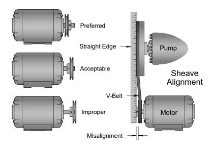
Equally important as tensioning is proper sheave alignment. The illustration to the far left shows how the sheave should be aligned on the shaft of the drive motor. The illustration, near left shows simple method for aligning the sheaves on the pump and motor.
