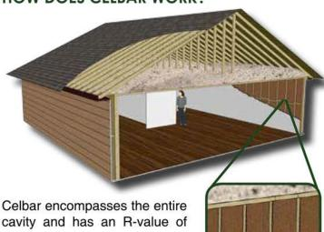
Celbar encompasses the entire cavity and has an R-value of 3.8 per inch. Celbar also stops air infiltration, keeping a cool house cool, and a warm house warm.
