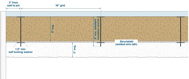
Cold Rolled: All longitudinal wires are cold rolled to a structurally designed shape.
